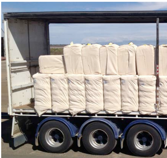
Arrangement with gap of greater than 300 mm at rear – place two bales face down across last two bottom rows and place a webbing restraint over the centre of the top bales
