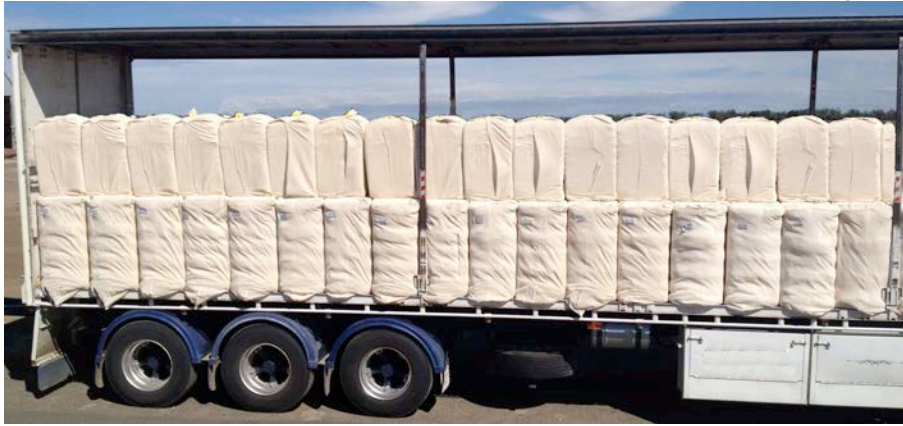
Base layer – three bales on end; Second layer 2 bales on side: Restraint over front row and then 1 for every four rows 6 webbing restraints for 120 bales
