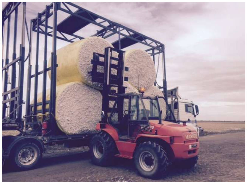
Photograph 2 – A trailer being loaded, showing end vertical rams and 45° check chains to same specification as tested semi trailer.
