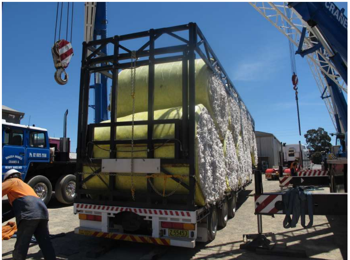
Photograph nine – Load after the three tilt tests. Also layout of tail board chains. Note vertical check chain is slack.
