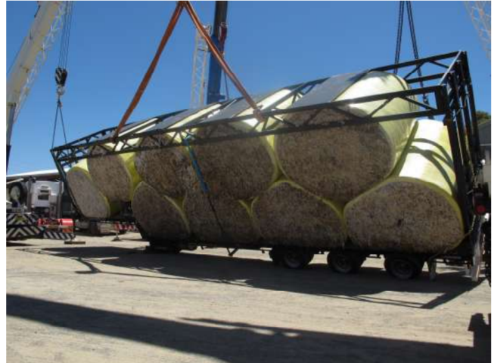
Photograph three – Detail of headboard showing vertical rams at corners and brace chain on support brackets. The vertical check chain in centre is redundant as the rams are fitted with self acting lock valves. Tailboard has similar arrangement.
