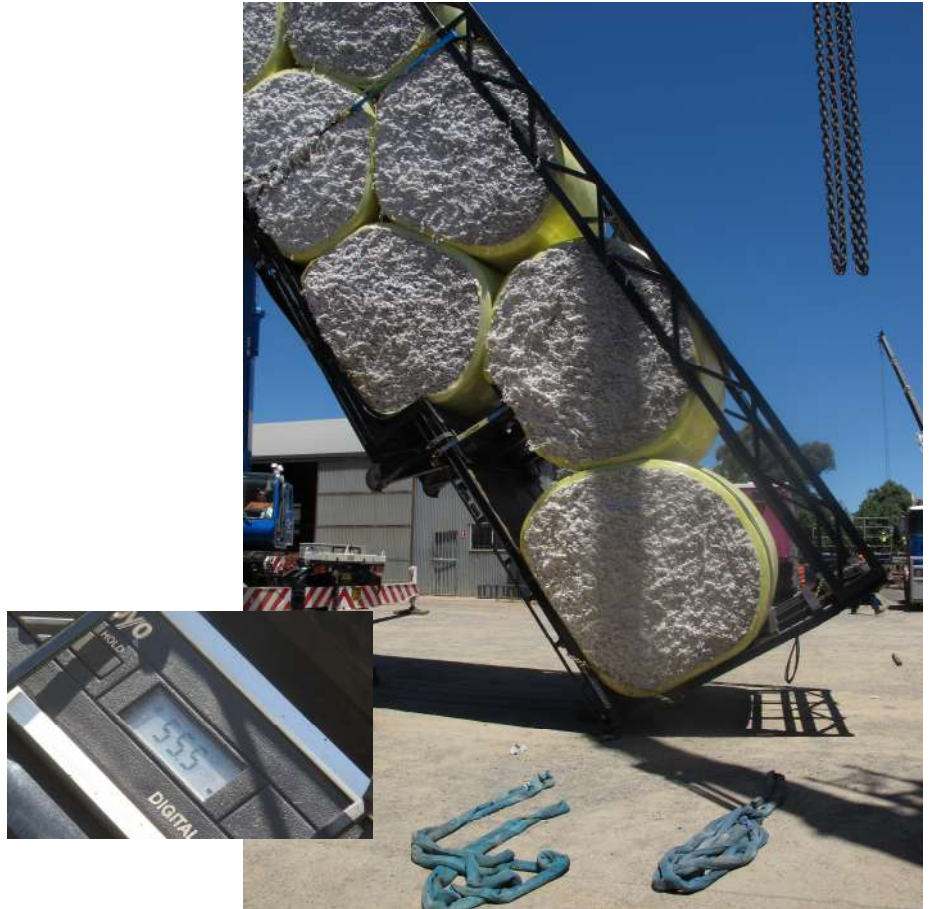
Photograph seven – Test two, forward tilt showing achieved angle of 55.5 degrees.
