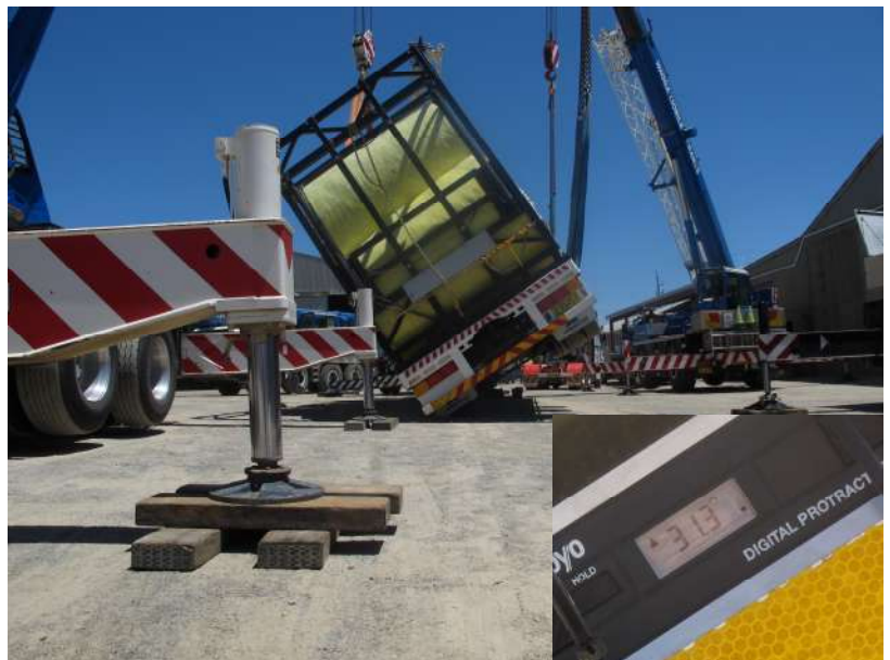
Photograph six – Test one, lateral tilt showing maximum angle reading of 31.3°
