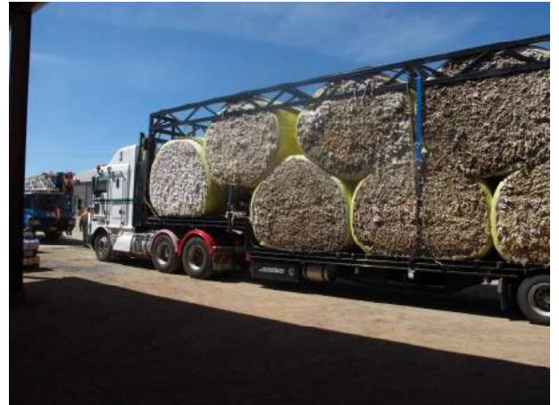
Photograph 1(b) Front detail of load of nine bales prior to tests showing drop deck and supported second bale.
