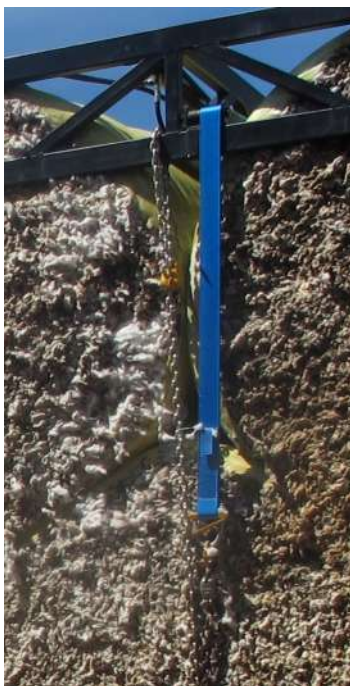
Photograph four – Detail of webbing strap at centre of trailer exerting downward force translated from horizontal ram at centre of frame.
