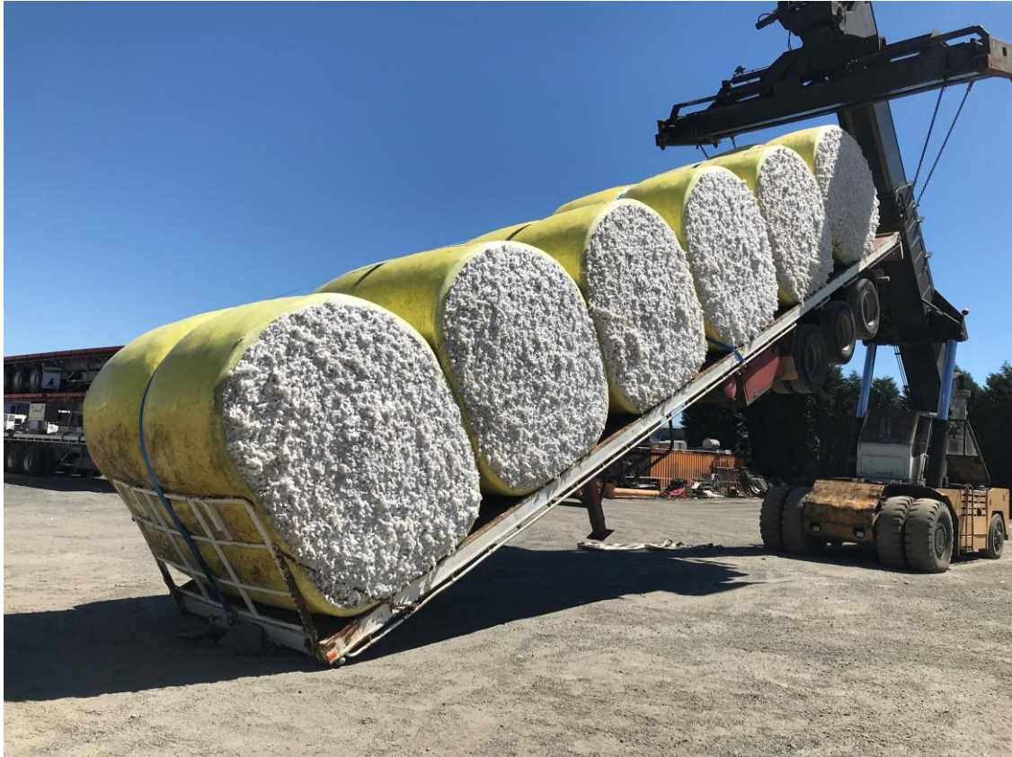
Image 5.1 – Longitudinal Forward; Note: test abandoned as headboard began to deform.
